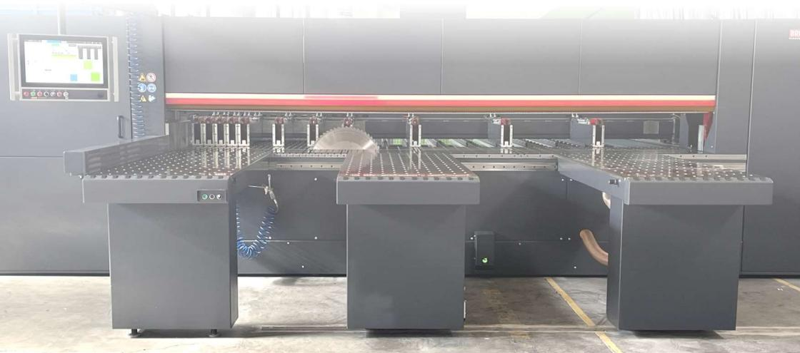
TAGLIO A DISCO DI PRECISIONE PER PIASTRE E LAMIERE DI ALLUMINIO DA 5 A 180 MM
