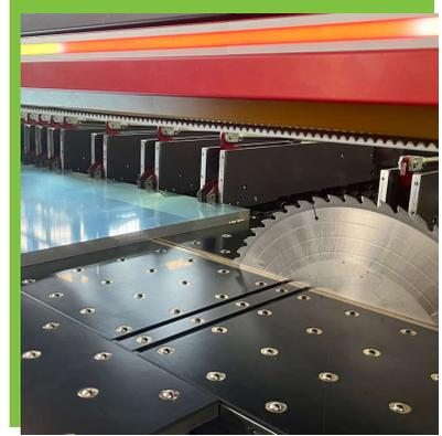
TAGLIO A DISCO DI PRECISIONE PER PIASTRE E LAMIERE DI ALLUMINIO DA 5 A 180 MM
